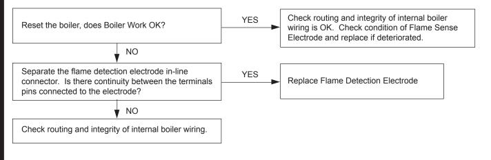
RESET PROCEDURE - To reset boiler, turn mode knob to reset position and immediately turn knob back to required setting.
