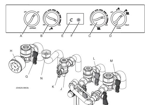
1. Check that the system has been filled and that the boiler is not IMPORTANT airlocked. Ensure the automatic air vent cap is open. Note.
